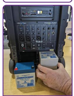
**6.** Place new batteries in compartment in same orientation that they were removed
