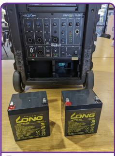
**5.** *Please Note:*Orientation of the battery terminals when removing exisiting batteries
